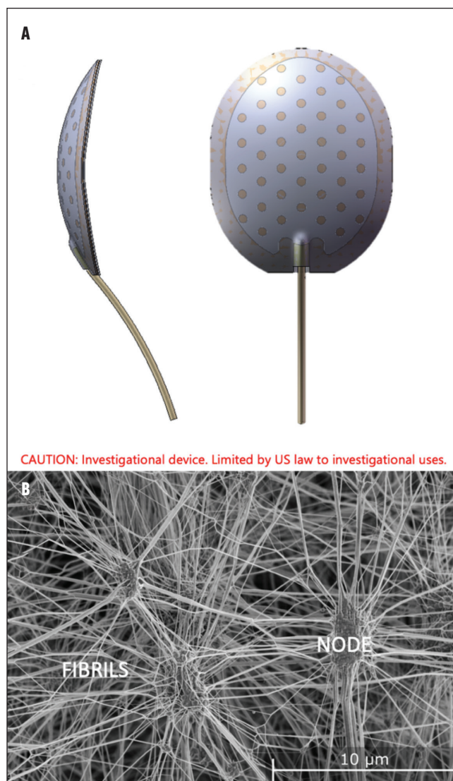
Figure 1. Gore ePTFE. Schematic of the investigational GDI prototype (A). Scanning electron microscopy of ePTFE (B). Varying arrangements of dense nodes and thin fibrils allow customization of the ePTFE membranes.
